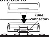
Select the dock insert for your Zune model from the table below and place insert in dock. Slide the Zune connector to left or right to match proper insert if needed. Never dock a Zune without an insert in place.
